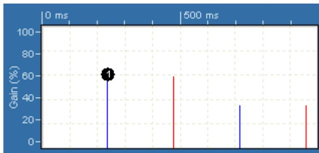
The blue mark shown above depicts the delay time for the left channel output, whereas the red mark depicts the delay time for the right channel output.
