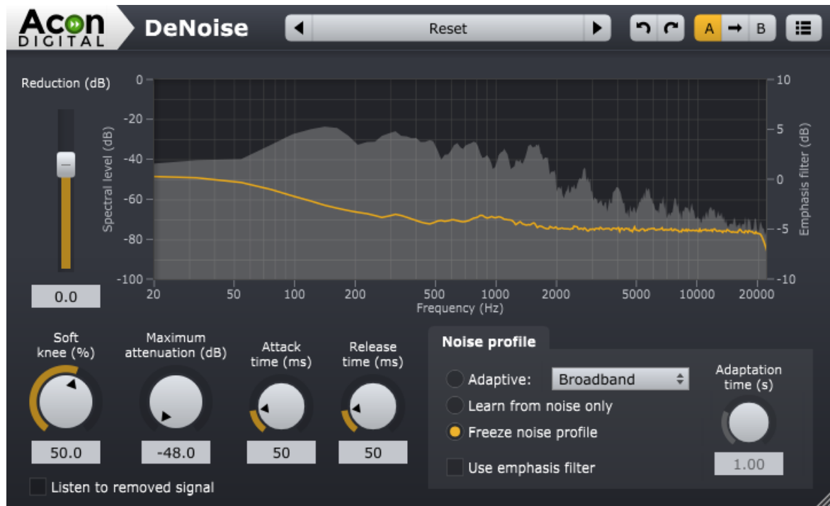
The DeNoise plug-in window. The graph shows the current noise profile as well as frequency spectrum of the input signal.
