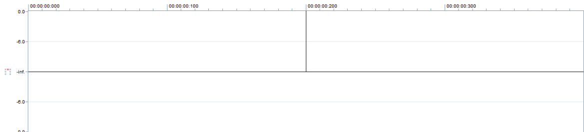
Input test signal consisting of a single pulse at 200 ms (Dirac impulse).
