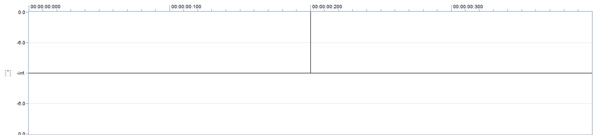
Input test signal consisting of a single pulse at 200 ms (Dirac impulse).
