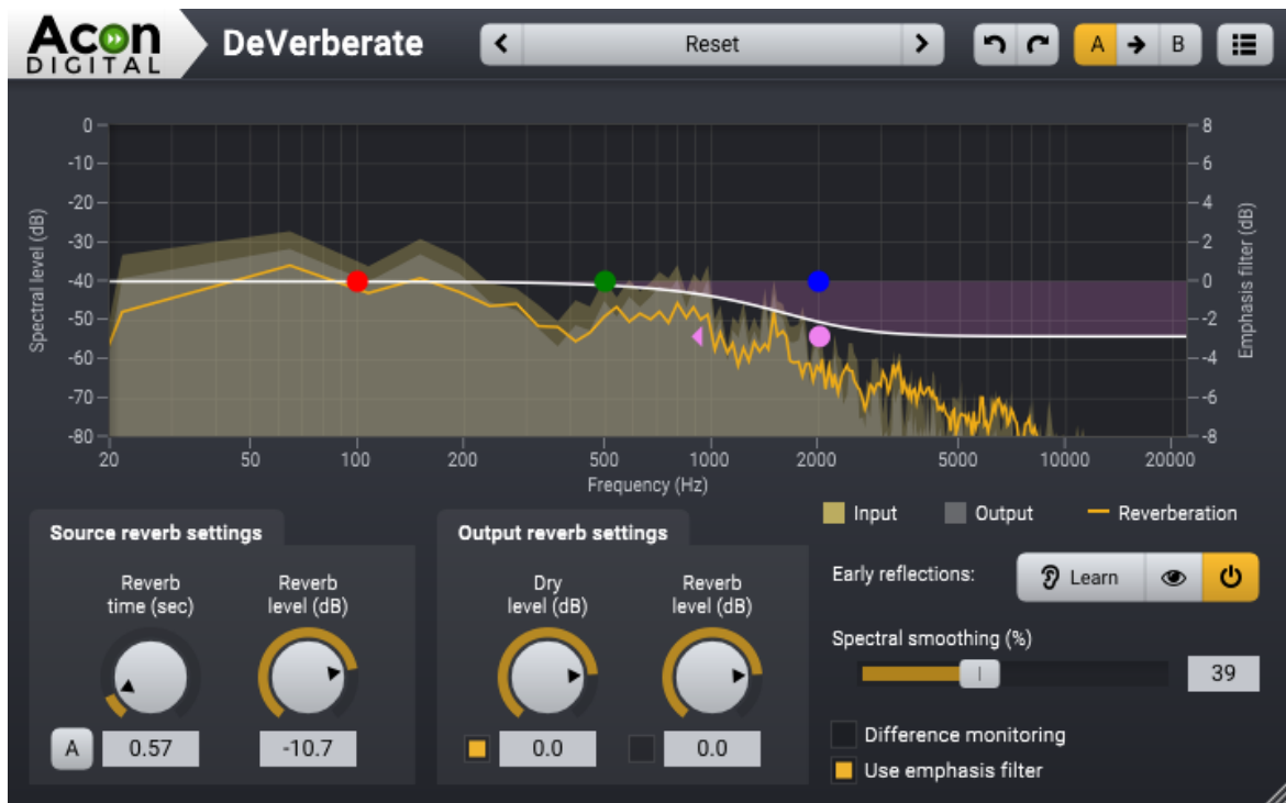
The DeVerberate plug-in window. The graph shows the estimated spectrum of the reverberation as well as frequency spectrum of the input and output signal.
