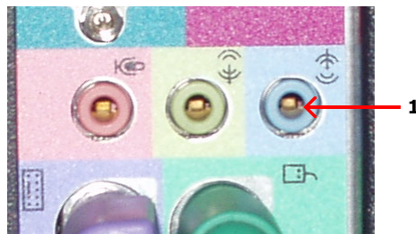
The back pane of a computer with an integrated sound card and a line in mini jack connector (1).
