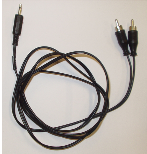
A connection cable with RCA connectors on one end and a mini jack connector on the other.
