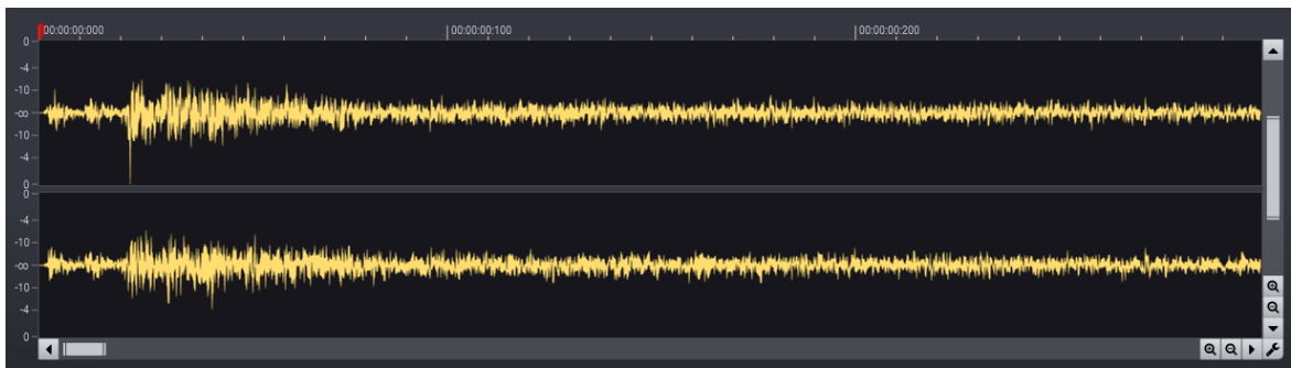
Results of an impulse response measurement of the Tokoy Hall preset in Acon Digital Verberate 2 (the first 300 milliseconds).
