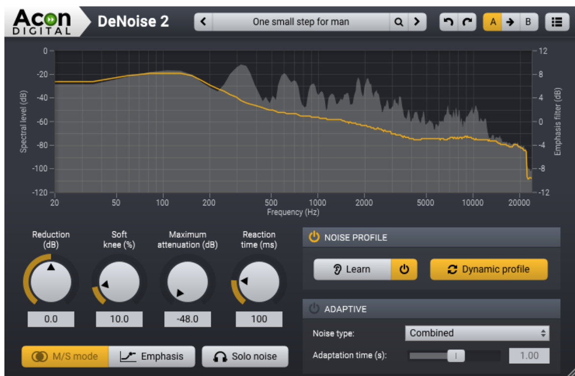
The DeNoise 2 plug-in window. The graph shows an estimation of the noise (yellow curve) as well as frequency spectrum (filled gray curve) of the input signal.
