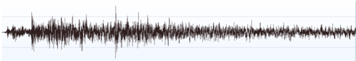
A measured impulse response from a real hall (the first 300 milliseconds).
